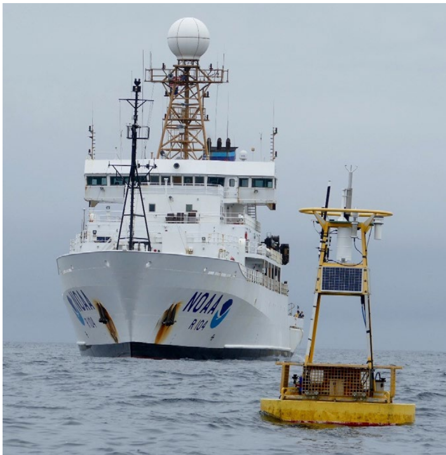
The NOAA research ship Ronald H. Brown taking calibration samples at the NANOOS Cha'ba monitoring mooring. Photo credit: R. Feely, Pacific Marine Environmental Laboratory/NOAA.
